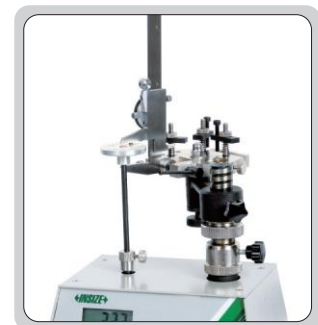
check the measuring force of calipers
