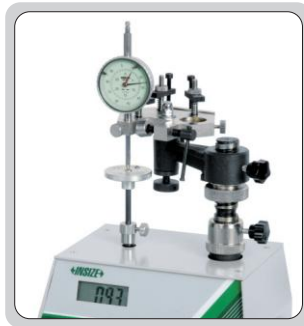
check the measuring force of dial indicators
